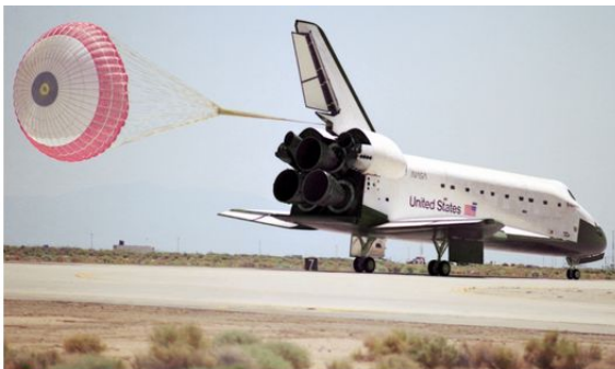
NASA Dryden Flight Research Center Photo Collection http://www.dfrc.nasa.gov/gallery/photo/index.html NASA Photo: EC92-05165-3 Date: 1992 Photo by: NASA STS-49 Landing at Edwards with First Drag Chute Landing
